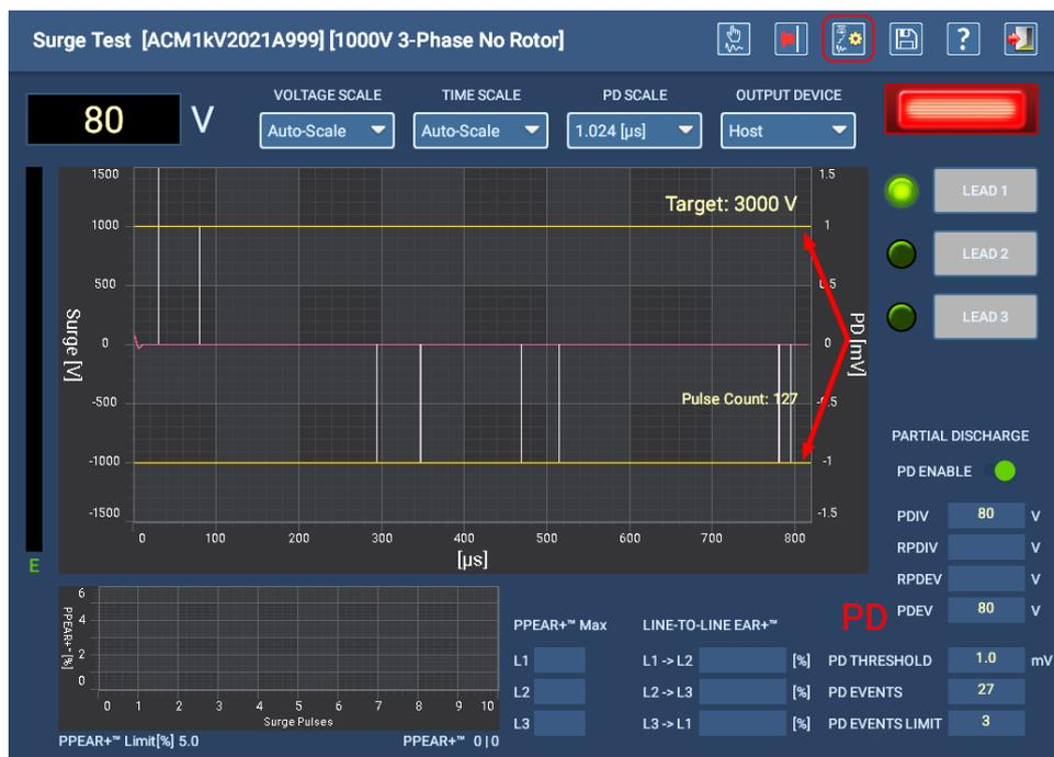
Fig 116: Surge Test screen in Manual mode for setting PD parameters.
