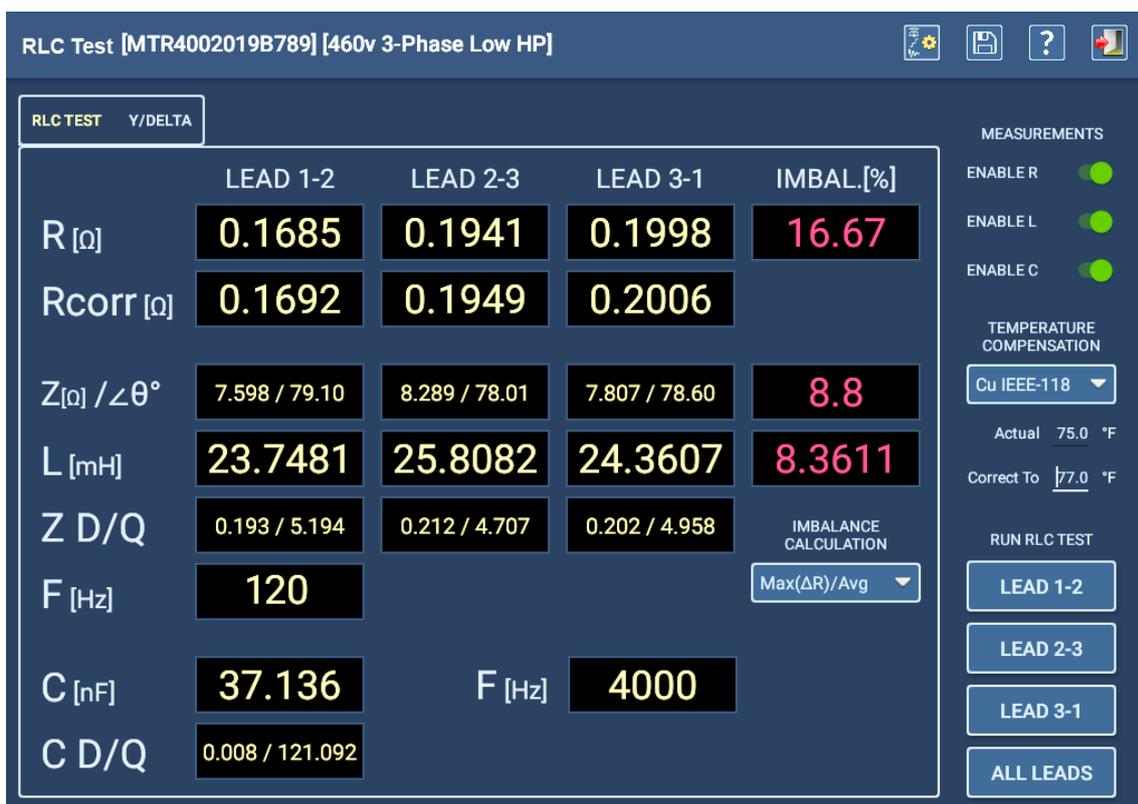
**Fig 81:** Manual Test—RLC main test results tab.
