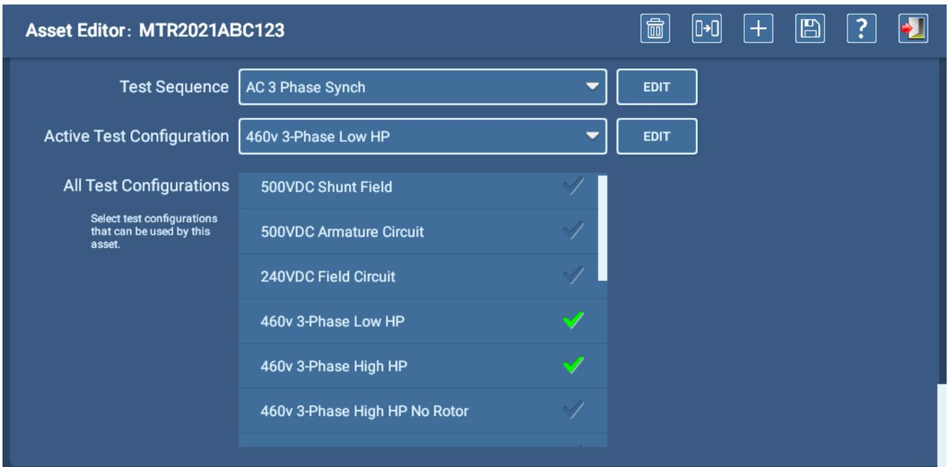
Fig 54: Asset Editor screen; selecting Test Sequence and Test Configurations.
