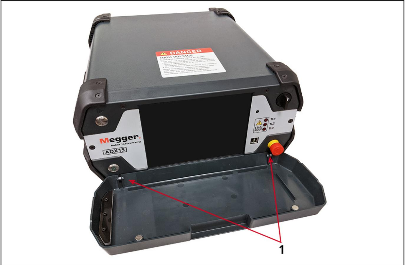
**Fig 21:** Locating hinge pins before removing the keyboard tray.
