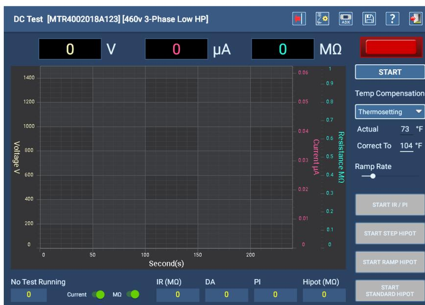
**Fig 83: Manual DC Test start screen.**
