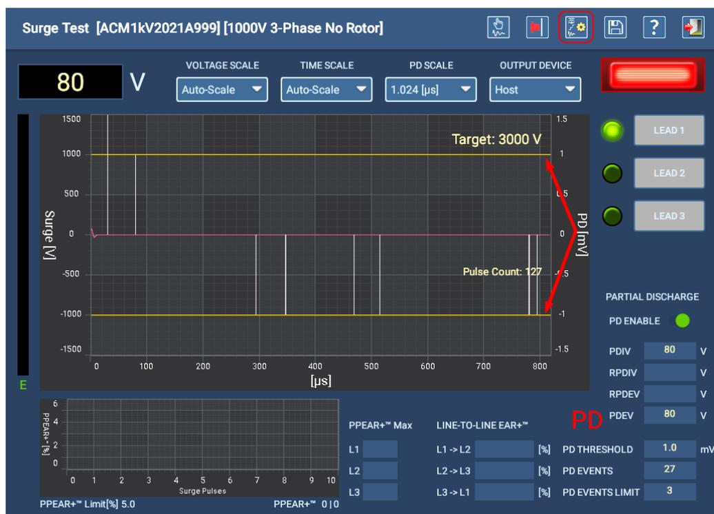
**Fig 117:** Surge Test screen in Manual mode for setting PD parameters.
