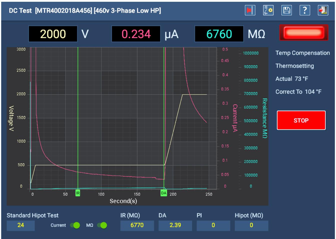
Fig 124: Auto DC Test screen—test in progress.
