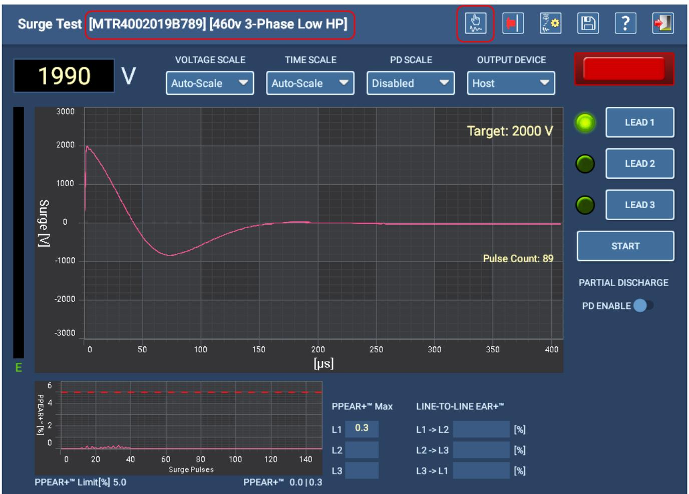
**Fig 89:** Acquiring reference waveform for Surge Test on LEAD 1.
