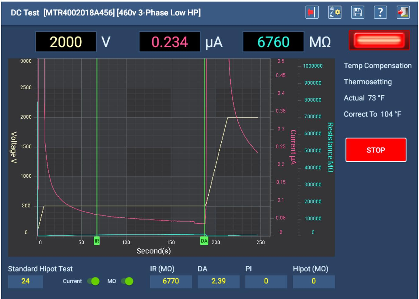
Fig 108: Auto DC Test screen running Standard Hipot Test.
