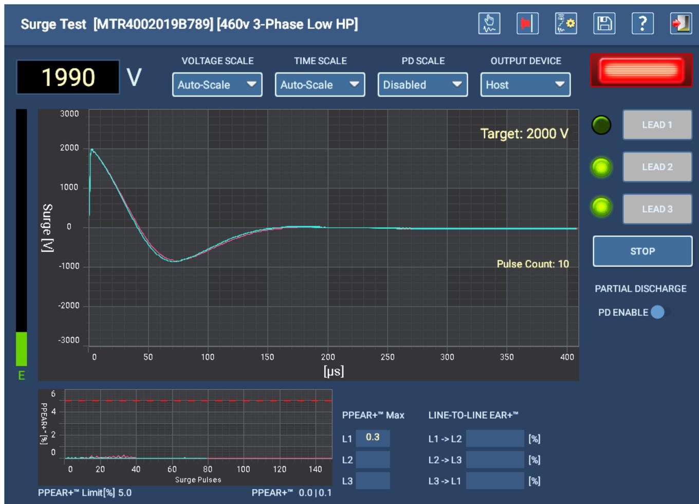
Fig 111: Auto Surge test screen—test in progress.
