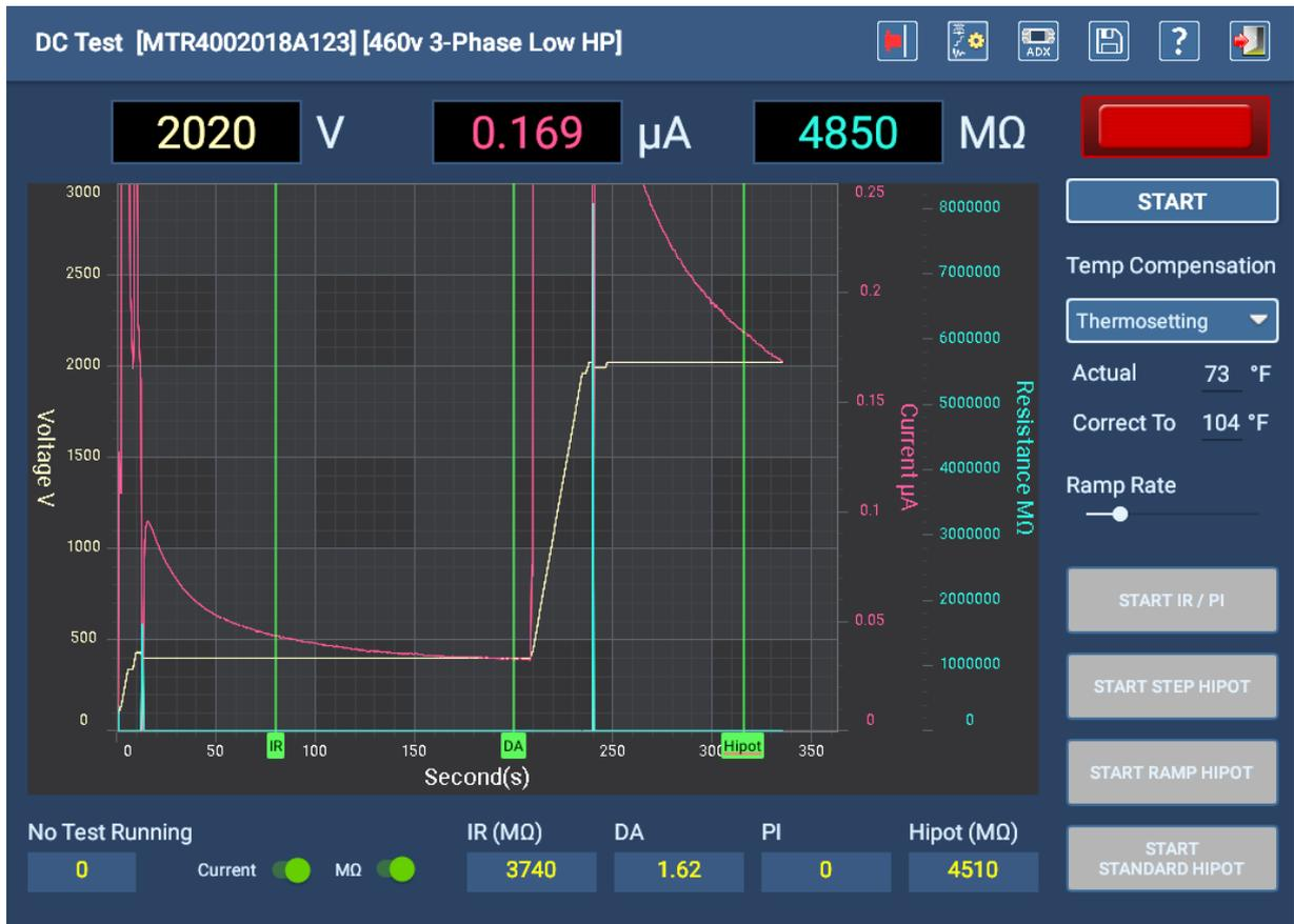
Fig 84: Manual DC Test screen—tests completed.
