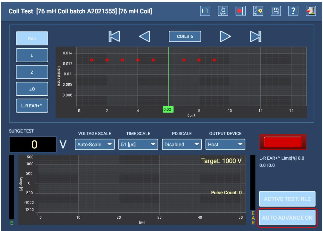
Fig 100: Coil Test screen with example RLZ test in progress.
