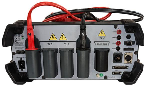
Fig 3: Inspect test lead receptacles and cables before each use.
