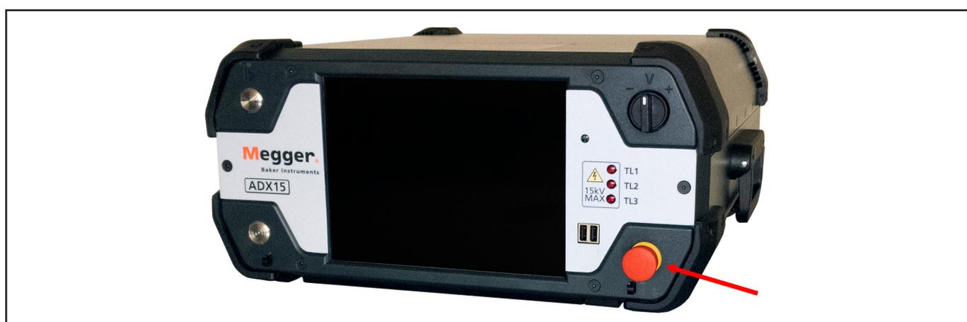
**Fig 145: Megger Baker ADX showing Equipment Stop button.**
