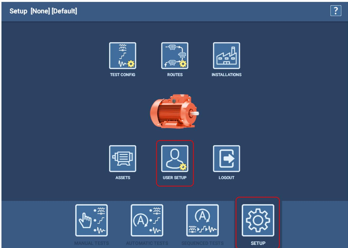
**Fig 29:** *SETUP* mode provides administrators with access to the User Setup screen.
