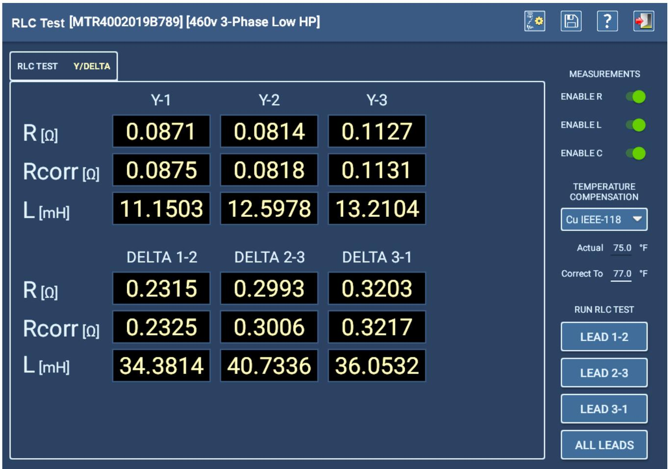
Fig 82: Manual Test—RLC Y/Delta tab.
