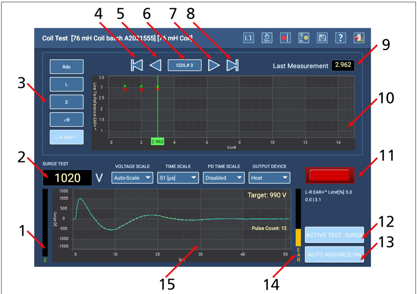
Fig 98: Coil Test screen elements.
